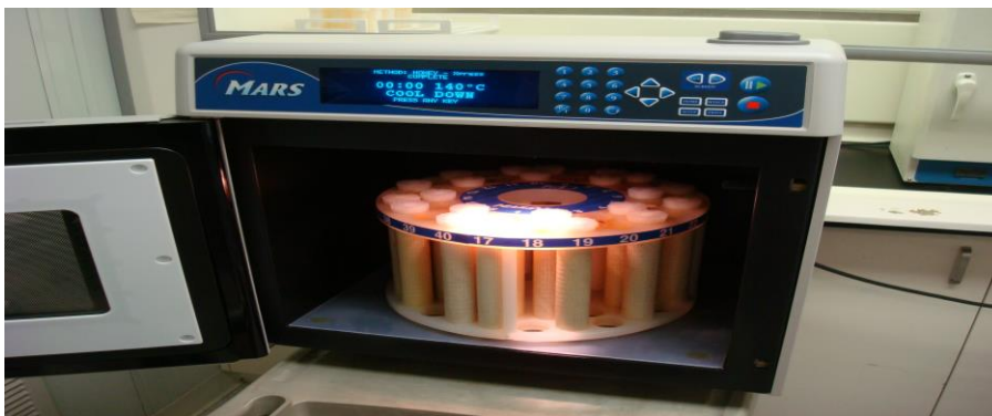
POWDERED SAMPLE ACID DIGESTED INTO “EXTRACT” FOR ICP/MS ANALYSIS
