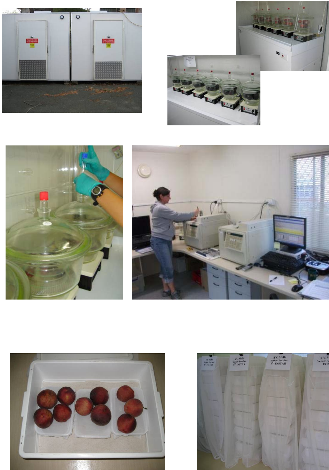
Figure 8 Methyl Bromide Most Tolerant Stage trials. Fruits containing infested immature stages of Medfly are exposed to a series of doses in glass desiccators at controlled temperatures 6 & 11 °C in separate fumigation rooms (top). Methyl bromide concentrations are monitored at 30 minute intervals throughout the trial period using gas chromatography (centre). After aeration, treated fruits are placed in plastic boxes and incubated for emergence of pupae at 26 \pm 1^\circ\text{C} ; 60-65% rh (bottom).
