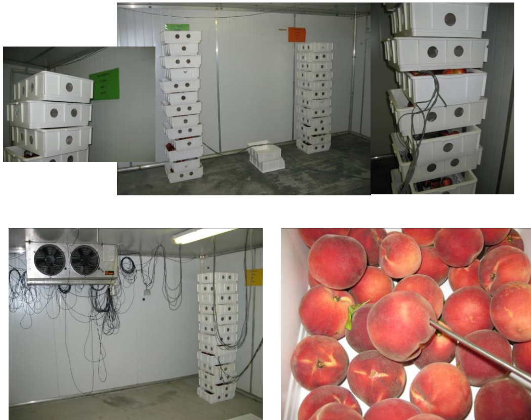
Figure 7 The plastic boxes (shown in Figure 6) containing immature stages in fruits are placed in 3 replicate cold rooms for exposure to 1°C or 3°C for conduct of the Most Tolerant Stage trials. Plastic boxes are removed from the cold room on designated dates after required period of cold exposure and returned to the incubation room to count survivors as pupae.
