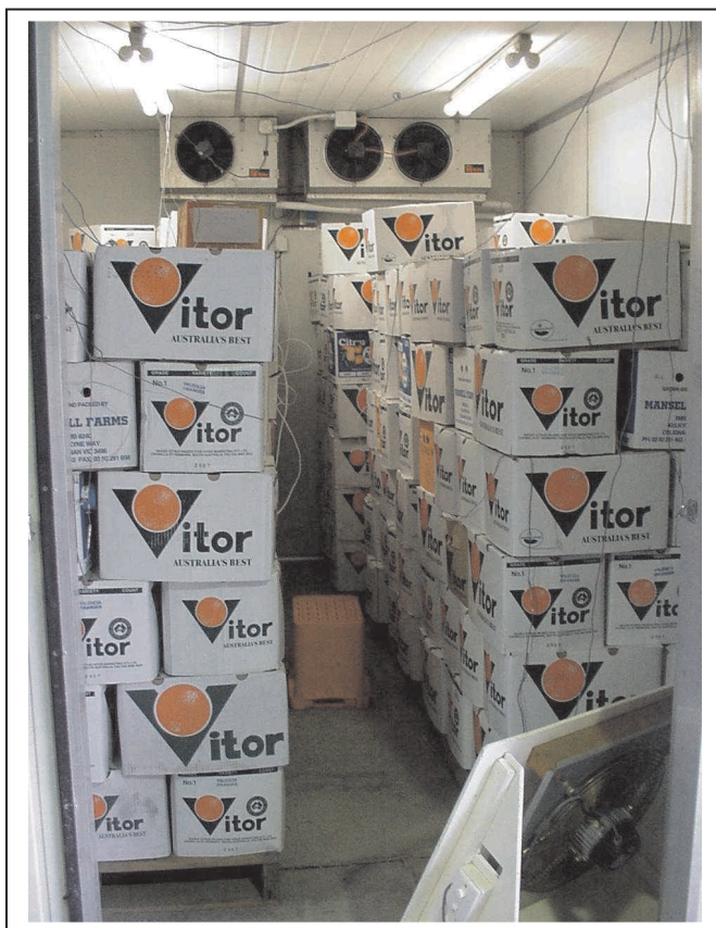
Figure 12 Filler fruit, apples in citrus cartons surround cherry cartons with infested cherries and non-infested cherries that are monitored for temperature (the temperature probe cables connecting the cherries to the data logger can be seen suspended from the ceiling).
