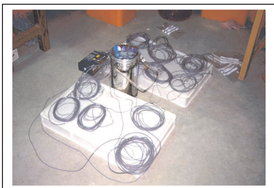
Figure 27 Squirrel Data Logger probes being calibrated in an ice/water slurry prior to treatment commencement.
