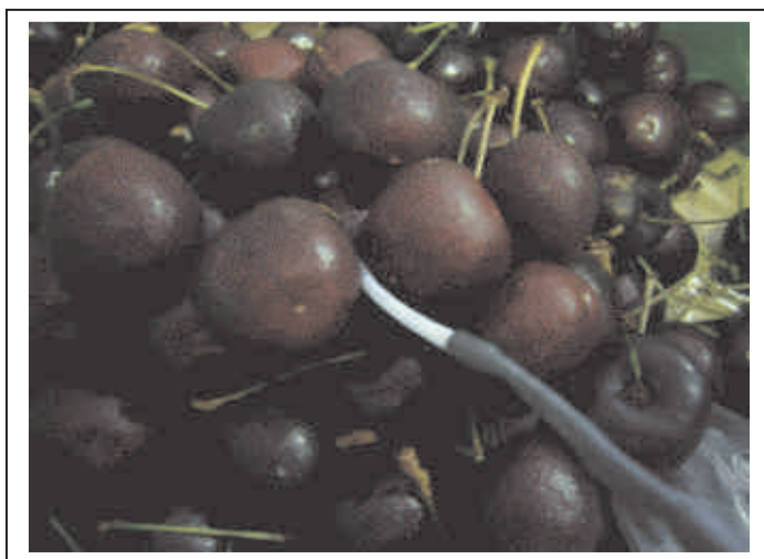
Figure 36 The data logger probes with the cherries attached were then placed in the centre of the carton and an attempt was made to pack other cherries tightly around the probe
