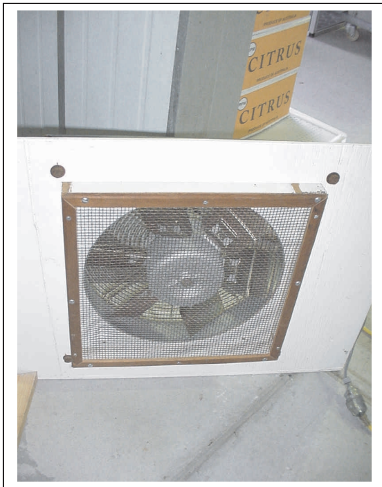
Figure 24 The front, bottom air circulation fan.
