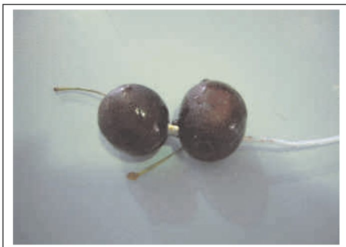
Figure 35 The data logger probes were inserted into two cherries alongside the stone.
