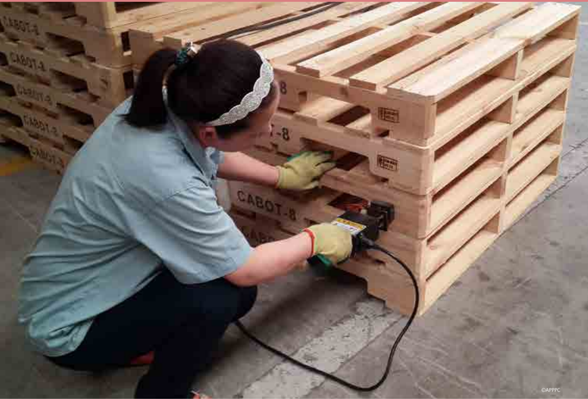
China — Implementation of the International Standard for Phytosanitary Measures No. 15 in practice-marking of wooden pallets.
