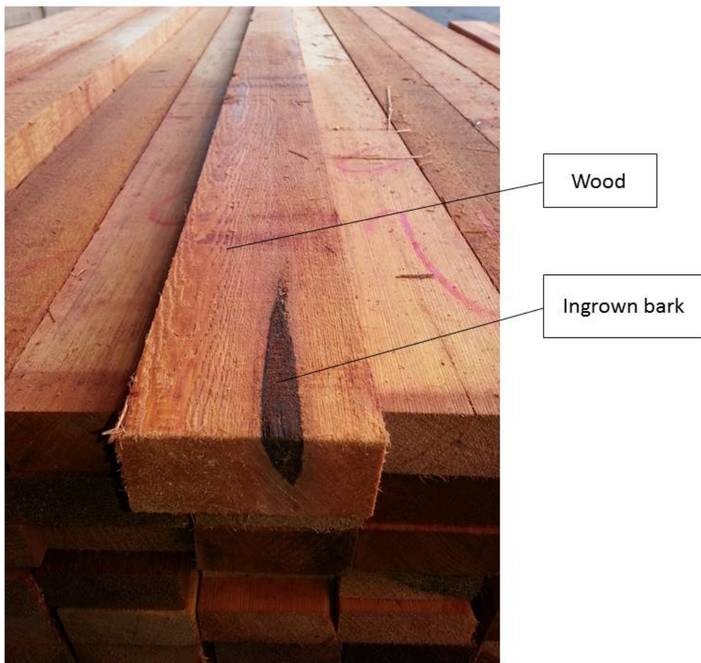
Figure 3. Sawn wood. Photo courtesy C. Dentelbeck, Canadian Lumber Standards Accreditation Board, Ottawa.
