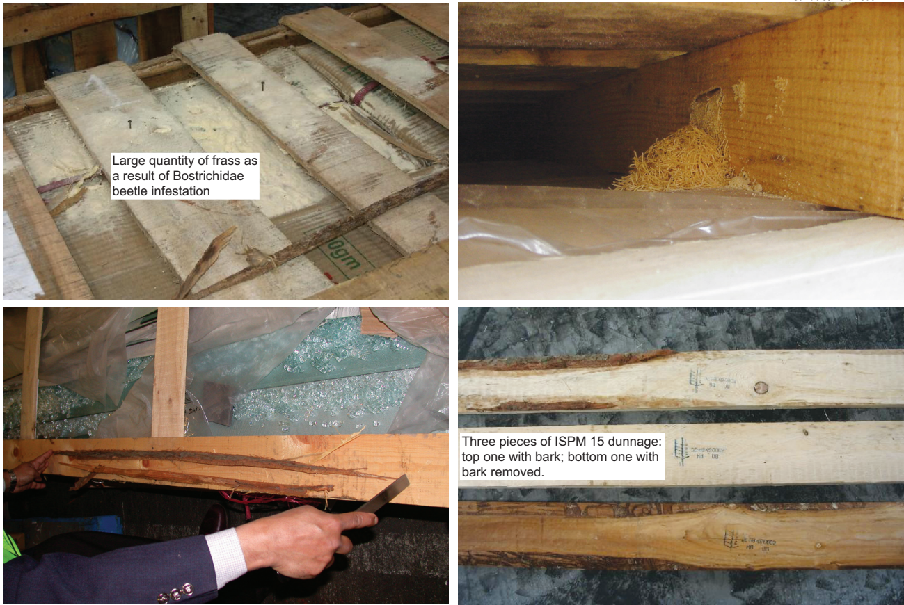
Figure 4. Examples of non-compliant SWPM encountered during the 2005 survey
