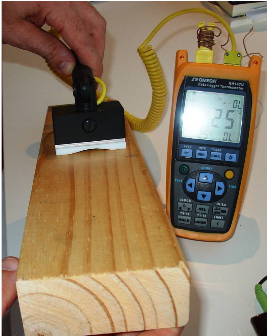
Figure 8: Illustration of proper application of handheld thermocouple useful as an auxillary measure to verify surface temperature of the SWPM after dielectric heating.
