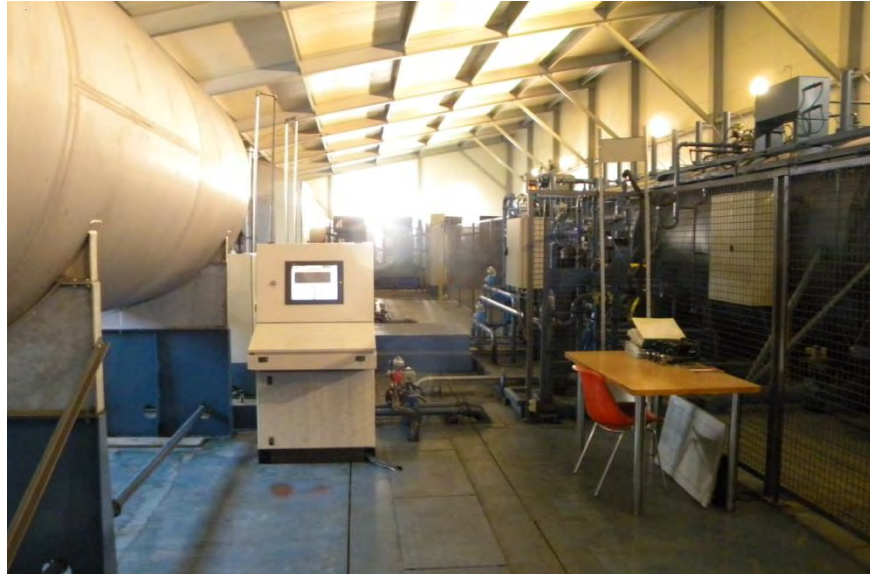
Figure 10. Wood impregnation plant. Chemical tanks are located on the left side of the picture. The pressure vessel is located on the right side of the picture
