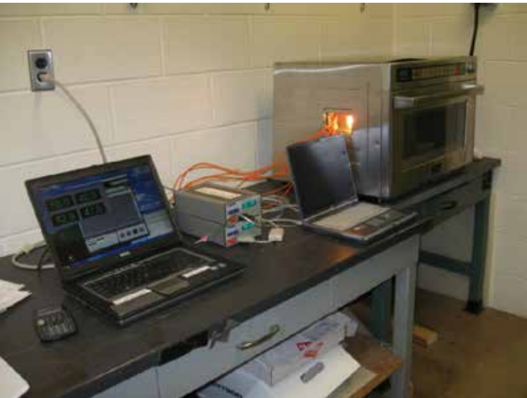
MW heating and recording of temperature of probes in-process
