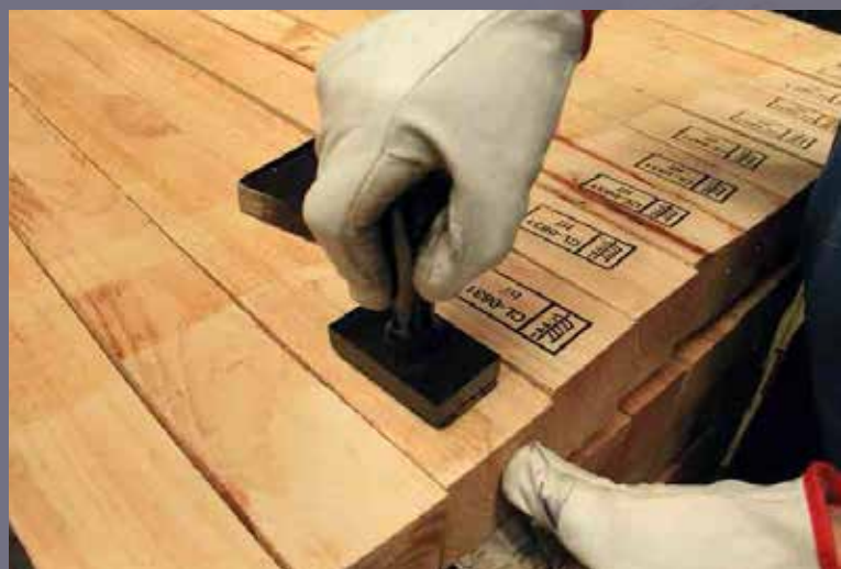
IPPC contributing to trade facilitation – The International Standard on Phytosanitary Measures (ISPM) 15 mark indicates that wooden pallets moved internationally are freed of wood boring pests.
